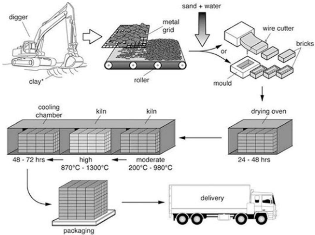
The diagram explains the way in which bricks are made for the building industry. Overall, there are seven stages in the process, beginning with the digging up of clay and culminating in delivery.
