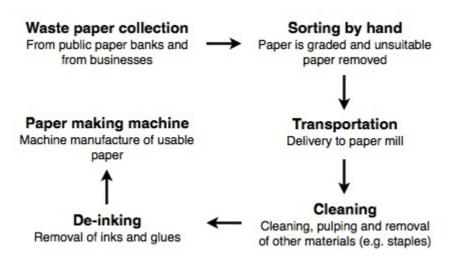
The flow chart shows how waste paper is recycled. It is clear that there are six distinct stages in this process, from the initial collection of waste paper to the eventual production of usable paper.
